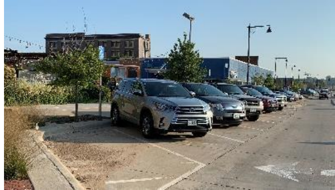
Figure 61. Front-out angle parking
